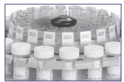
Load filters—open end up Load vials and slides—
